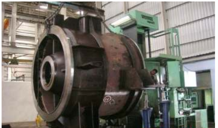
Tubular Kaplan Casing Being Machined on WOTON CNC HBM
