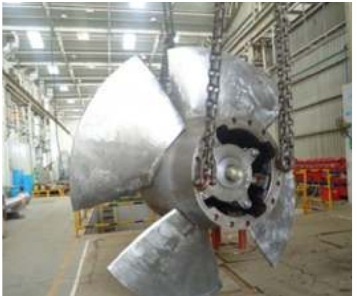
Assembly of Kaplan Runner of Ranni Perunad at works 2X2MW HEP
