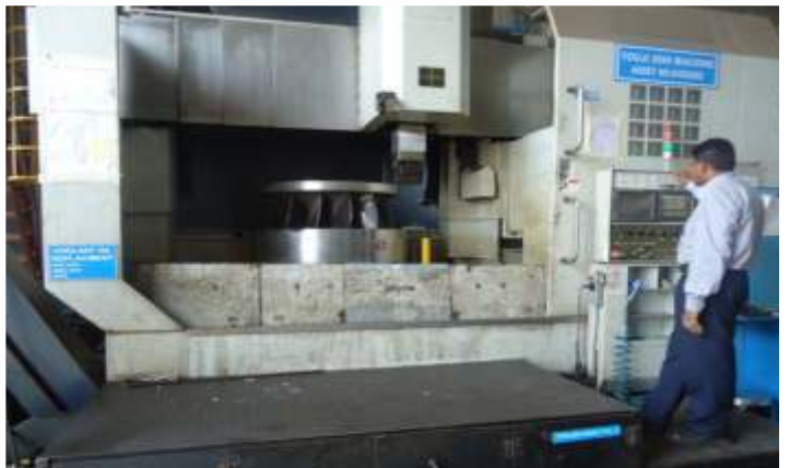
Francis Runner machining on CNC VBM
