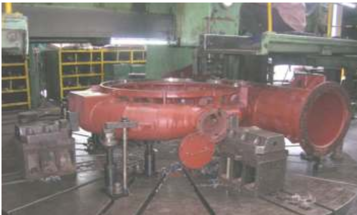
Francis Spiral Casing machining on SK 40 VTL.
