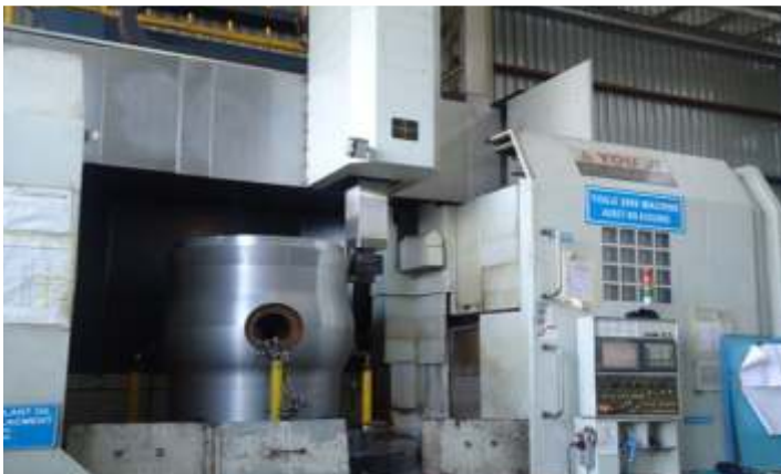
Kaplan Runner Hub machining on CNC VBM.
